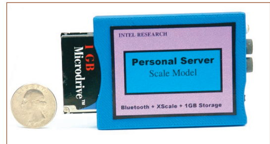
Figure 4. Intel Research's Personal Server, a prototype system that combines powerful processing, high-density storage, and a Bluetooth radio.
