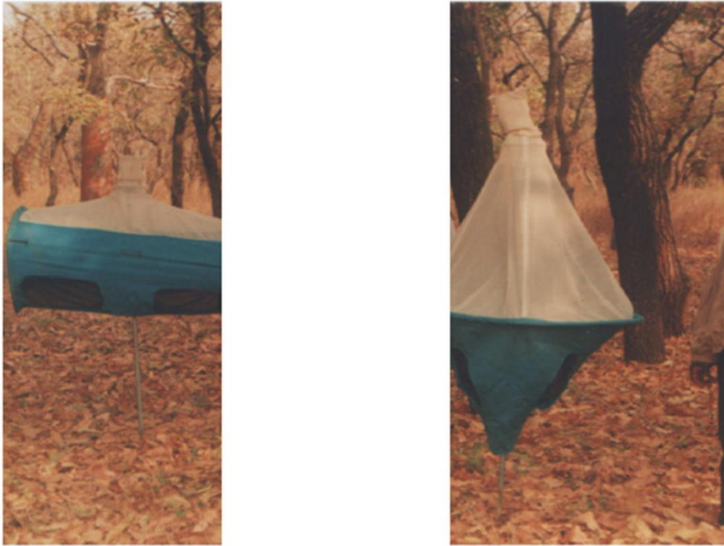
Plate 1. Drum-shaped and biconical-shaped traps for tsetse flies (Seifert, 1996).
